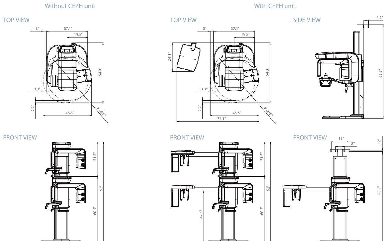
**\*An additional 3 inches (76.2 mm) of space is required behind the unit for wall mount bracket installation (mandatory unless there is a base mount installation).**
