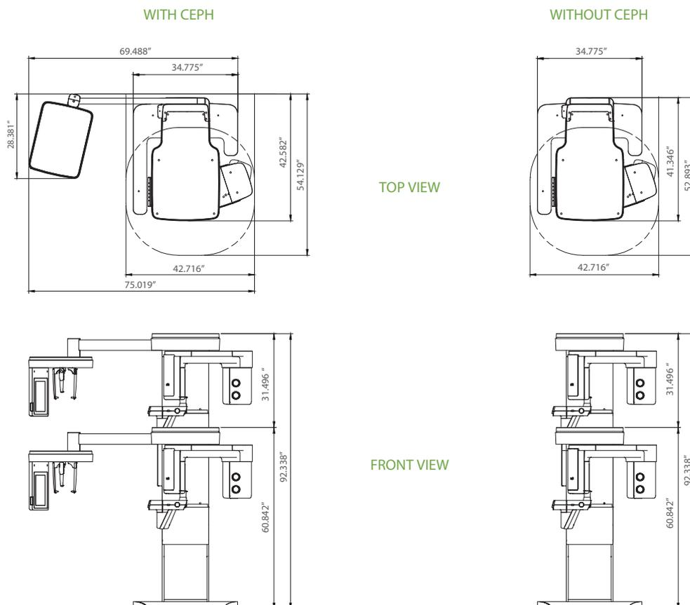
**\*An additional 3 inches (76.2 mm) of space is required behind the unit for wall mount bracket installation (mandatory unless there is a base mount installation).**
