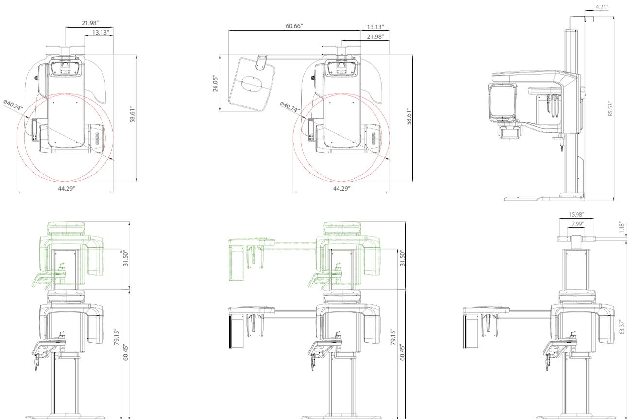
**\*An additional 3 inches (76.2 mm) of space is required behind the unit for wall mount bracket installation (mandatory unless there is a base mount installation).**
