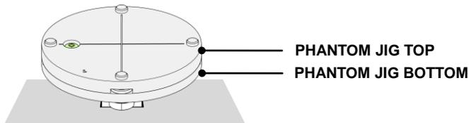
3. Make the PHANTOM JIG ASS'Y level by using BUBBLE LEVEL and three ALIGN PINS.
