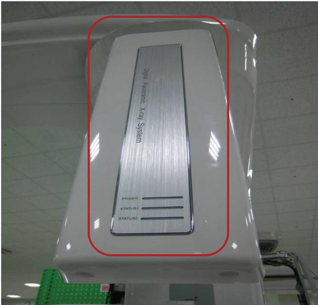
2. Detach the outer cover of the rotating unit. The outer case can be disassembled by removing 4 Truss bolts from the top and bottom of the casing, as illustrated below.
