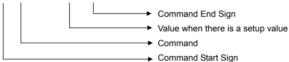
Ex: **[SPM\_HV\_\_0800]**: Tube Voltage Setting Command
