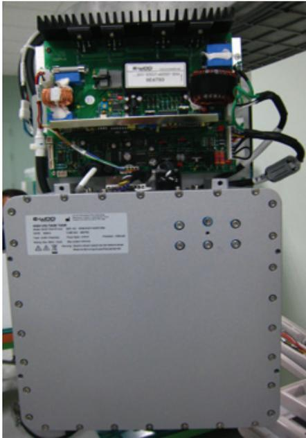
5. Disconnect the board first. Then undo 4 screws for grounding, which are located at both sides of the board.
