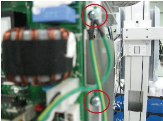
6. Disconnect cables CN105x2EA and P1013A, and the cable from the X-ray tube.
