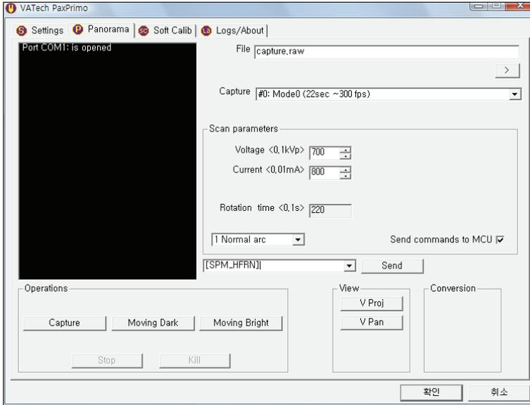
7. If you want to manually make micro adjustments to the HALF position, set the desired value using the command **[SPM\_HFST\_0000]**. When moving the Central area to the right, raise the hfst value; and when moving to the left, adjust the value down.
