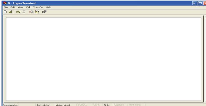
If there are strange characters or trash-like contents that appear on the terminal, they are caused by incorrect setup. In this case, check whether the same **Com Port** is being used by the equipment and the Hyper-terminal, and check the cable conditions as well. If the set up is not correct, you will likely not be able to use the Key Board input. In this case, changing into a different communication speed is one of the troubleshooting methods.
