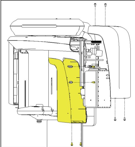
4. Take the 6 rubber caps off, and then remove the 6 Truss Bolts. Then loosen the screws and detach the upper cover of the Rotating Unit, as shown in the figure.
