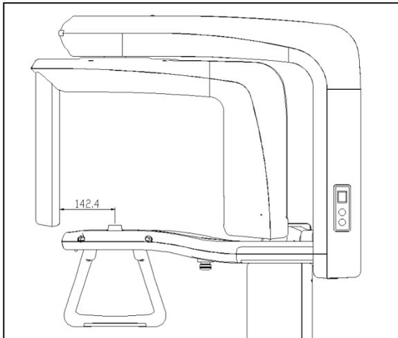
3. Loosen the fixation wrench bolts of the chin rest block. Then, taking into account the measured distances, adjust the bilateral distances at 15.4cm.
