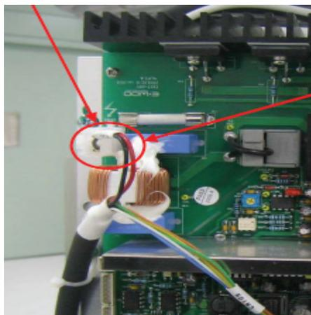
Important: Disconnect the cable from the Board.
