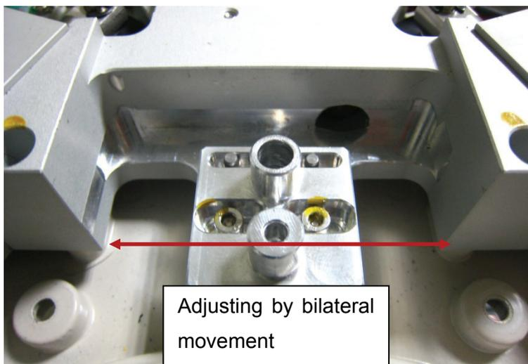
4. Using a wrench, tighten the loosened chin rest block. Repeat correction procedure 11.1. After which, if the resulting value is within the error range, finish the adjustment of bilateral distance values of the chin rest block.
