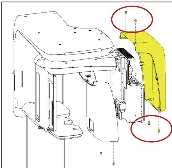
3. Detach the inner cover of the Tube head of the Rotating unit.
