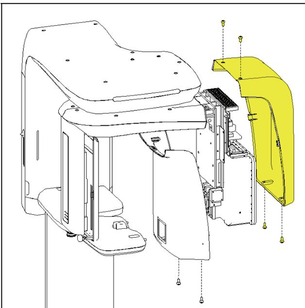
3. Take the 2 Truss bolts off the bottom of the inner case of the rotating unit; then detach the case by removing 4 more bolts from inside the case.
