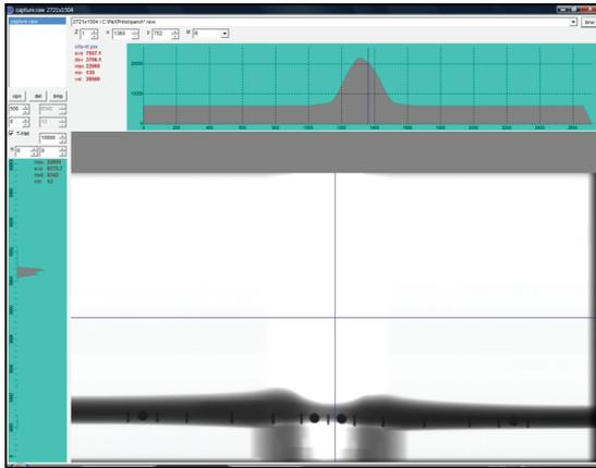
17. Enlarge the image, if necessary, by increasing the Z value.
