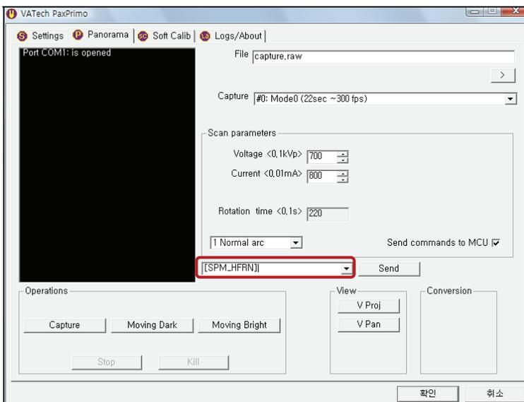
5. Input **[spm\_hfrn]** in the command input field, then the unit will automatically move to the Half value position stored in its memory.
