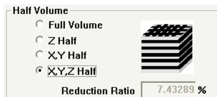
Reduction by half along X, Y, and Z axes, respectively
