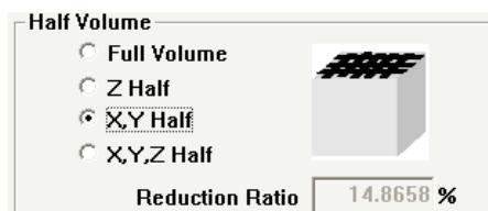
Reduction by half along X and Y axes
