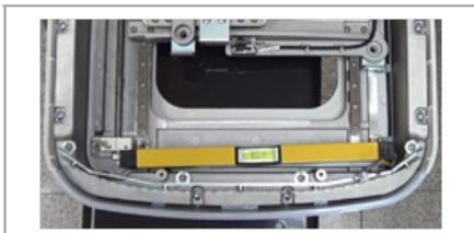
2. Turns each of the four screws on the base left and right until the bubble in the spirit level comes to the middle. The location of each screw is circled in the image below.
