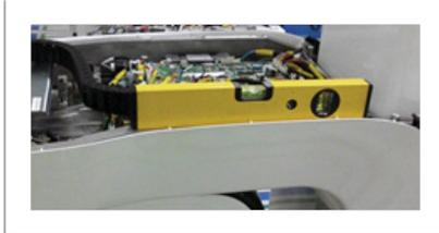
2. Adjust the screws until the bubble of Spirit Level centers (level) by turning the front and/or back screws clockwise or vice versa.
