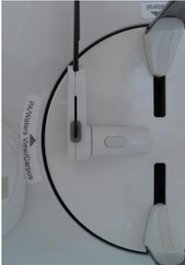
2. Fold the nasal positioner up. The nasal positioner is not used in Waters View mode.
