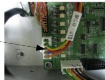
3. Connect MCU CN19 cable into the CN19
