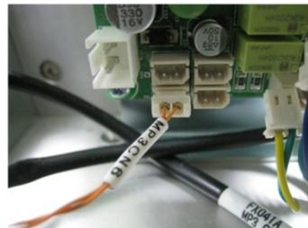
5. Tie the cables with the cable tie (**Part No.:5**) together.
