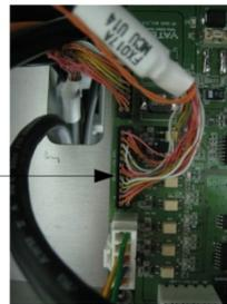
2. Connect FX017A MCU CN18 into the connector CN18
