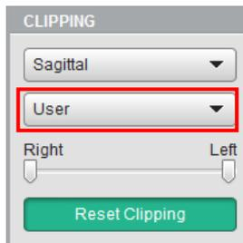
4. Drag the slider and the image will be clipped in the selected direction.
