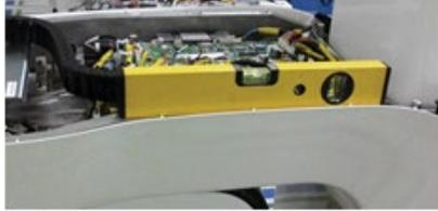
2. Adjust the screws until the bubble of Spirit Level centers (level), by turning the front and back screws clockwise or vice versa.
