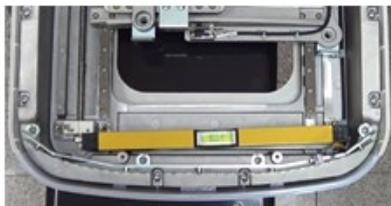
2. Adjust the base until the bubble on the Spirit Level centers in the middle, by turning left and right screws clockwise or vice versa.
