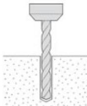
3. Remove the debris and clean the holes using the dust pump.
