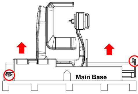
6. Put the **Main Unit** with the **EPS (Main Base)** on a Transport Dolly and move it to the installation site.
