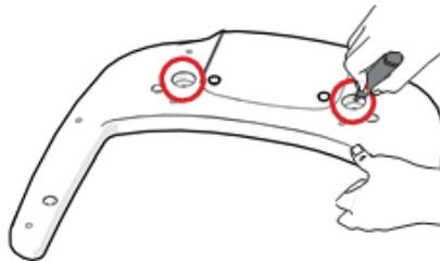
2. Drill the floor holes of size 12mm x 30mm (depth) using the concrete hammer drill.
