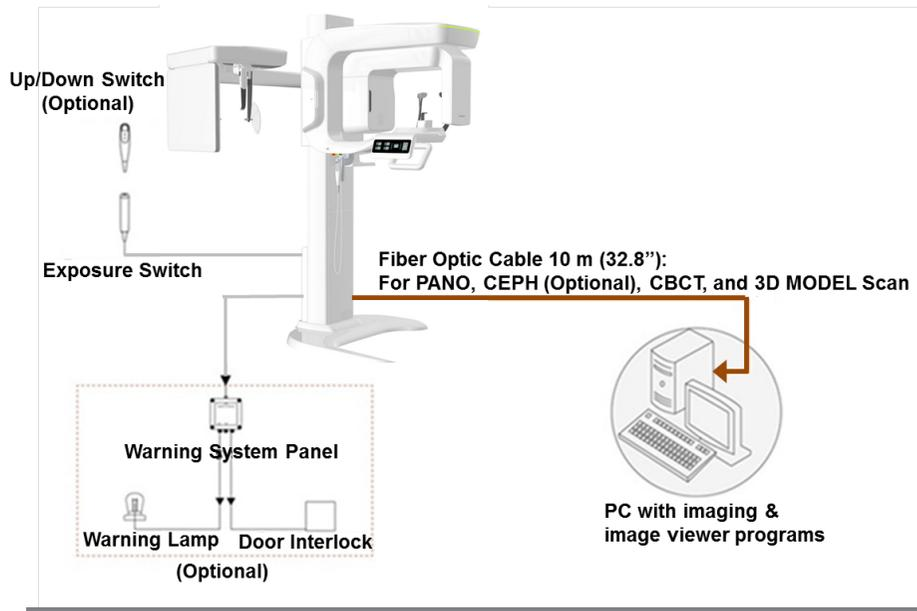
**Fiber Optic Cable** - Used to transfer image data to the PC.
