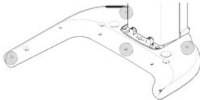
3. When the leveling is completed, make sure that all eight set screws touch the floor by turning them clockwise if necessary.
