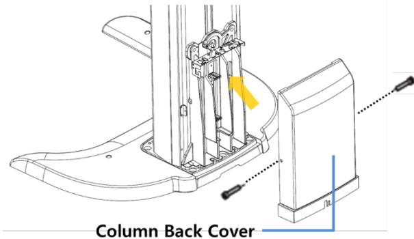
3. Ensure the cables go through the Column Back Cover holes as shown in the figure.
