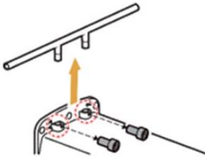
2. Put two wrench bolts into the holes on the bottom of the column unit.
