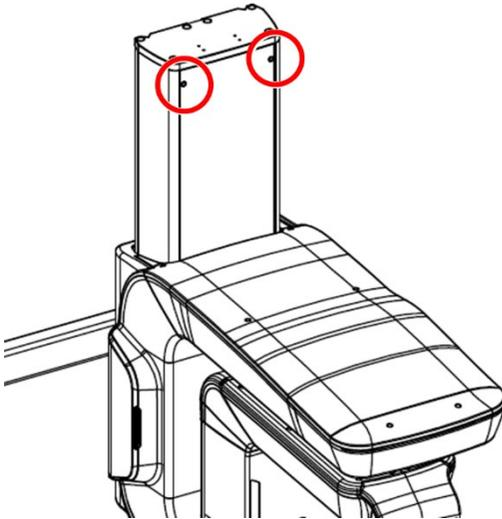
3. Remove the Column Rear-Top Cover as shown in the figure.
