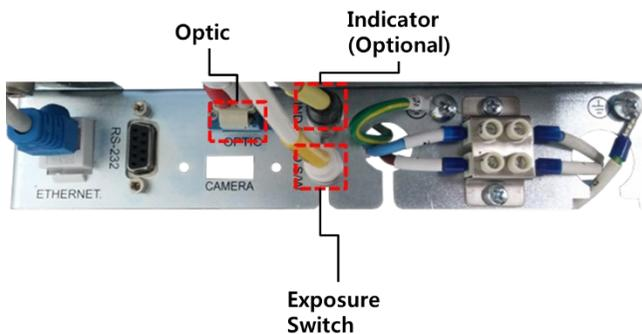
Use the Cable Tie (Part No. 20) to fix the cables as shown below after the connection is completed.
