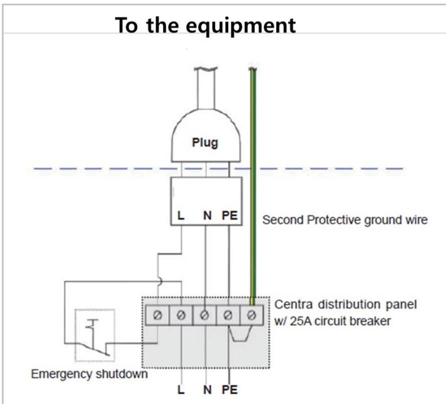
1. The cable sizes: N, L, and PE  $\geq$  12 AWG (3 x 4 mm<sup>2</sup>).
