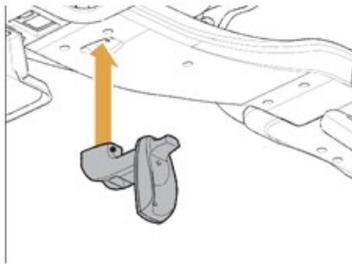
2. Connect the UP/DOWN switch to the unit and hang it on the UP / DOWN Switch Holder
