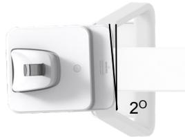
1. Push the Chinrest attachment part on the handle frame towards the machine until the end of the Chinrest attachment part is printed in "-PANO-" silk. Push until you hear a "click" sound.
