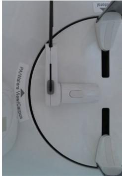
2. Fold the Nasal Positioner up. The Nasal Positioner is not used in Carpus mode.
