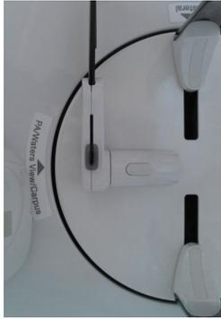
2. Fold the Nasal Positioner up. The Nasal Positioner is not used in PA mode.
