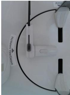
2. Fold the Nasal Positioner up. The Nasal Positioner is not used in Waters' view mode.
