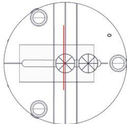
3. Insert the PHANTOM JIG BOTTOM into the Chinrest and then put the PHANTOM JIG TOP on the PHANTOM JIG BOTTOM.
