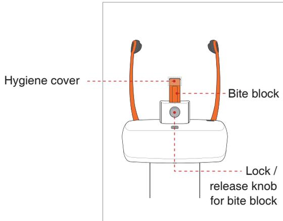
A. Insert the bite block into the Chinrest receptacle on the equipment.
