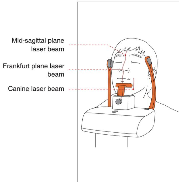
**A. Mid-sagittal plane laser beam:** Position the Mid-sagittal plane laser beam at the center of the patient's face to prevent magnifications of the left or right side in the final image.
