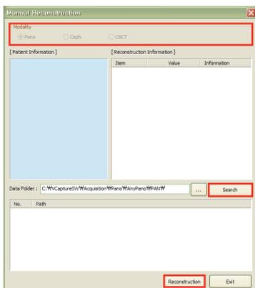
If automatic reconstruction of the image fails, use this function to reconstruct the image manually. Select **Modality** and click **Search** → **Reconstruction**.
