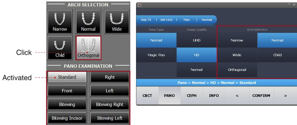
**Orthogonal:** This mode enables overlapping regions of teeth to be minimized when acquiring images in the ROI. If orthogonal arch is selected, its sub-modes are activated.
