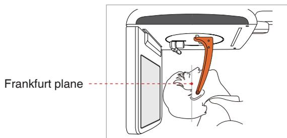
F. Place the ear rods along the patient's ear canals. Make sure that the ear rods are comfortably, yet firmly in place.
