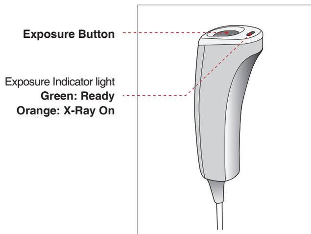
The exposure switch allows the operator to control image acquisition from outside of the X-Ray room. Press and hold the exposure switch down until acquisition is complete. Premature release of the exposure switch will abort image acquisition.
