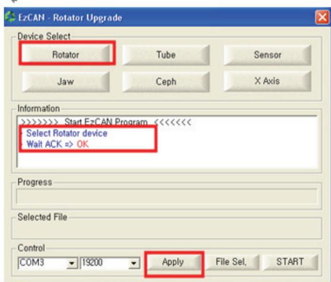
2. Select Rotator from Device Select. Thereafter, if the communication with the equipment is successful, “**Wait ACK=>OK**” will appear after a few seconds on the Information window.
