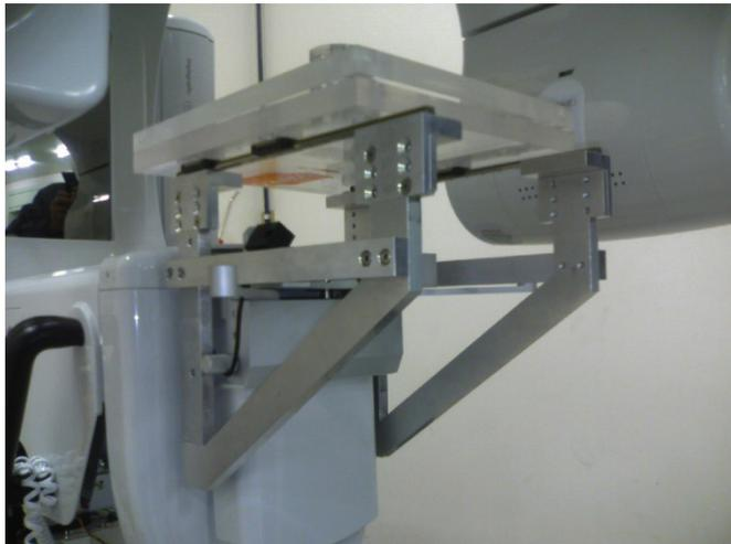
[Example Photo of CT Phantom Mounting on Implagraphy Equipment]
