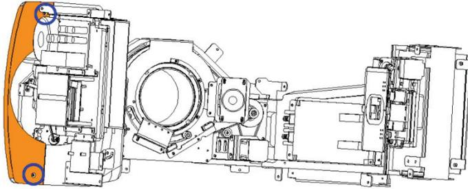
14. Remove 4 bolts, and then disassemble Case H.
