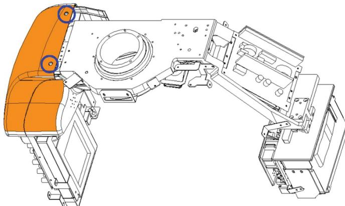
13. Remove 2 bolts, and then disassemble Case G.
