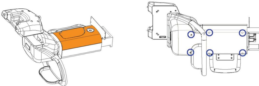
3. Remove 4 bolts, and then disassemble Case B.
