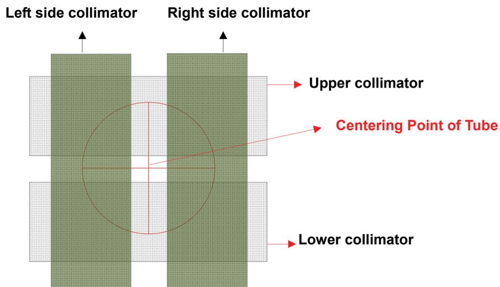
The unit is 0.1 mm that is the distance of collimator's actual movement. The base of all collimators is the center, and its value is 0. Set the distance being alienated from the center in positive number unit. When it is negative number, the collimator moves in opposite direction (Necessary for Panorama)
