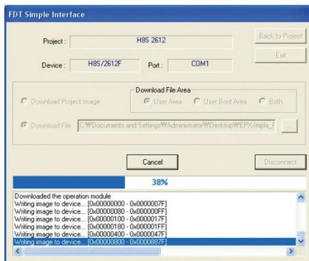
11. After the uploading of X-axis MCU new firmware is completed, select **'Disconnect'** button.
