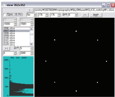
As shown in above figure, set the difference of each window level as 1, and as changing the level, confirm on the proper threshold value that shows all of 8 beads on one slice.
