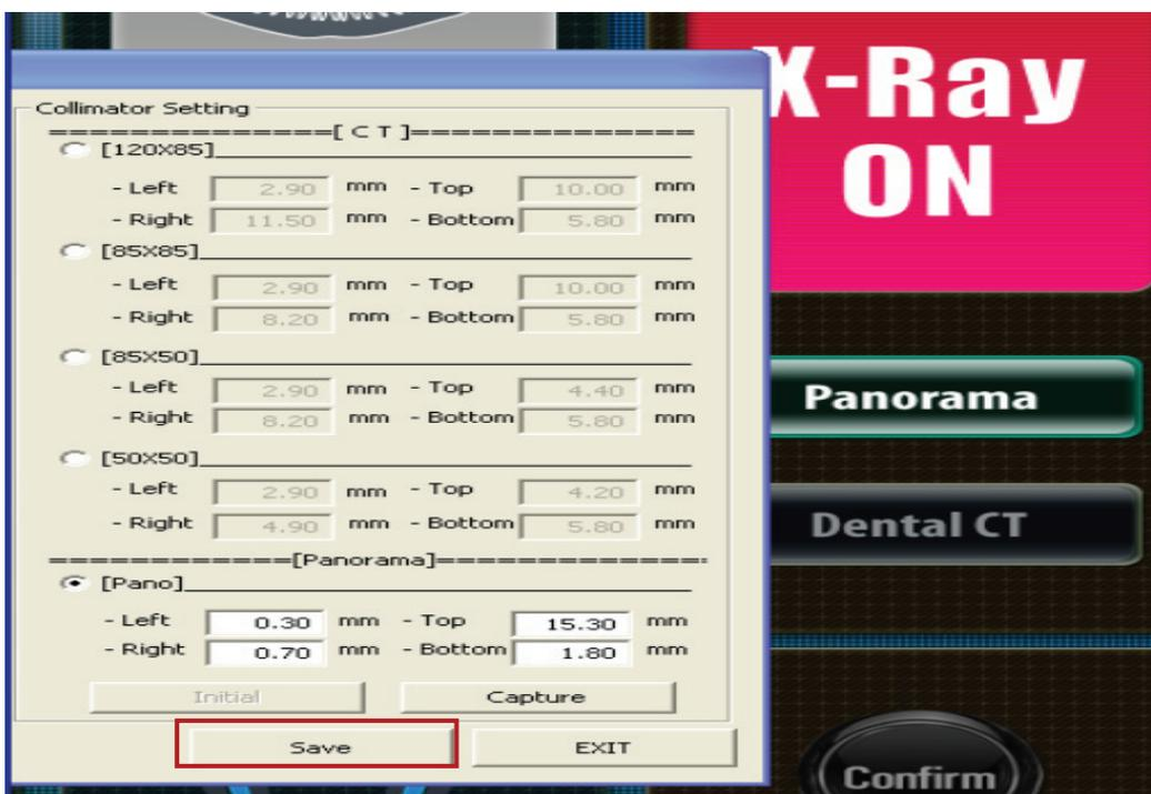
As shown in above figure, when the Collimator setting is completed, press the “save” button to save the values.
