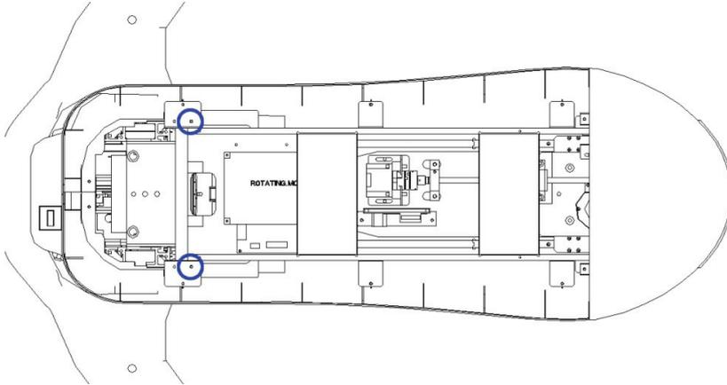
6. Turn 2 bolts and the horizontal beam adjustment bar to remove them, and then disassemble Case F.
