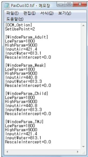
**For WindowParam16 adult section, scan the CT Phantom in the Adult Mode, and the average values of each measured substances, that are air and water, should be recorded. Also, for WindowParam16 child, scan CT Phantom in the Weak Mode, and the average values of each measured substances should be recorded for use.**
