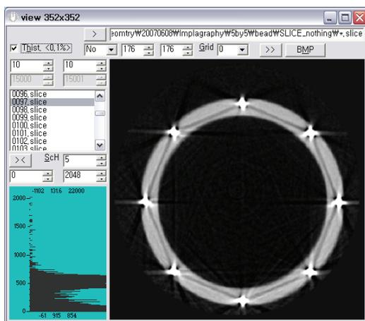
If Bead is appeared in the form of letter U, this indicates that DETOFFSETYY is not optimal, therefore adjust the value and perform the reconstruction again.
