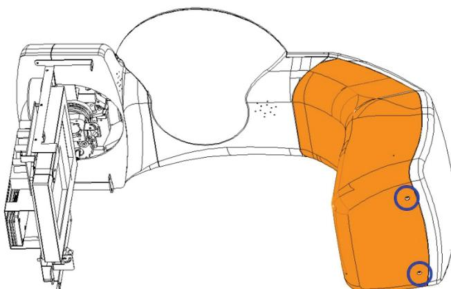
9. Remove 4 bolts of each direction respectively, in total of 8 bolts.
