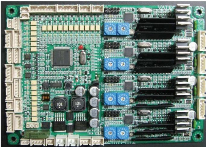
3. Turn DIP Switch No.1 on X-axis Board to the position of “On”.
