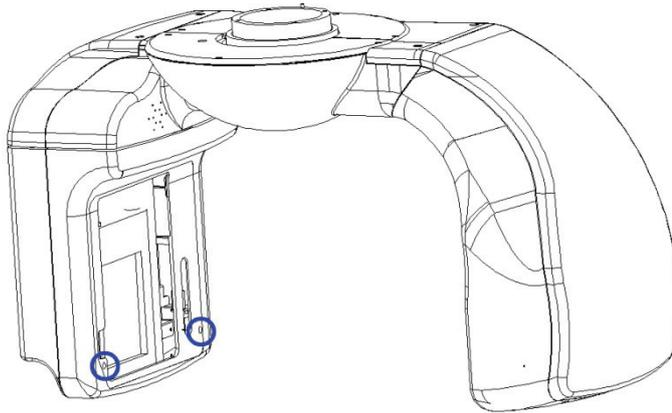
3. Turn the sensor part slightly and remove 1 bolt that is hidden.
