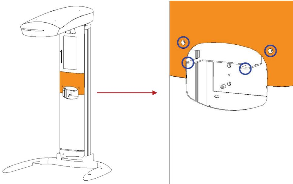
2. Remove 4 bolts, and then disassemble Case B and C.
