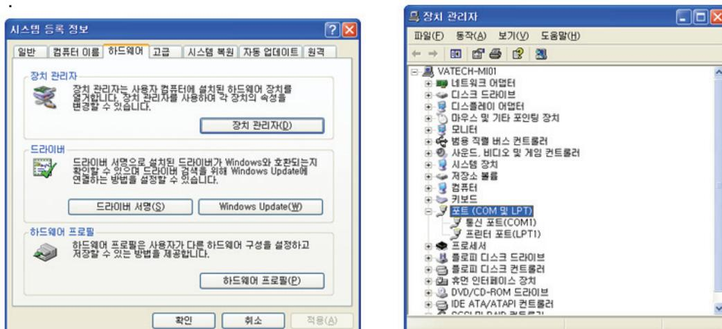
5. Check and select the communication port between the equipment and the computer (=Comport).
