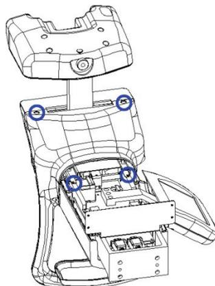
4. Remove 2 bolts, and then disassemble Case C.
