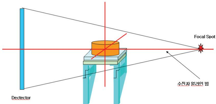
[Figure 2. Drawing for Align method after mounting CT Phantom Jig]
