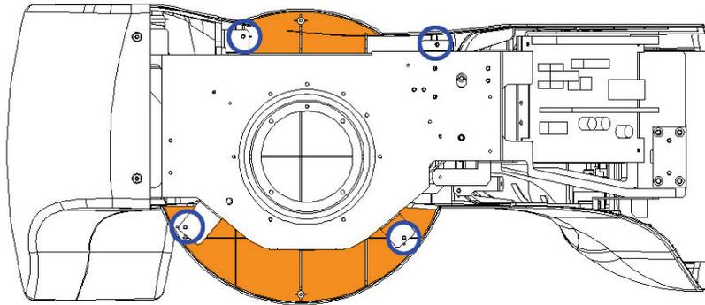
11. Remove 6 bolts, and then disassemble Case F.
