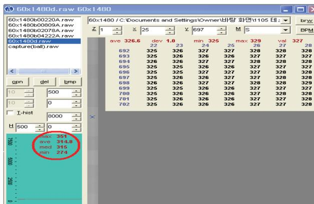
4. When clicking **'Bright'** from **Soft Calib** Tab, the command is sent automatically and when **Vapan** window is activated and by pressing the irradiation switch for about 1 second, the applicable bright data is to be acquired.
