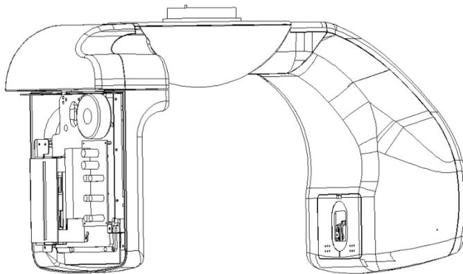
6. Remove 4 bolts, and then separate Cover B as shown in the following Figure.
