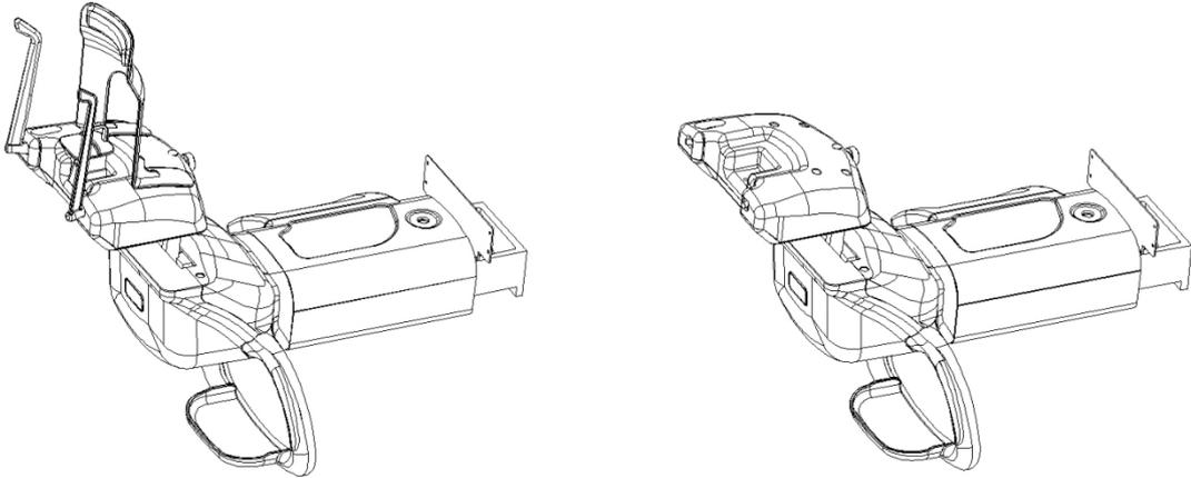
2. Remove 6 bolts, and then disassemble Case A.
