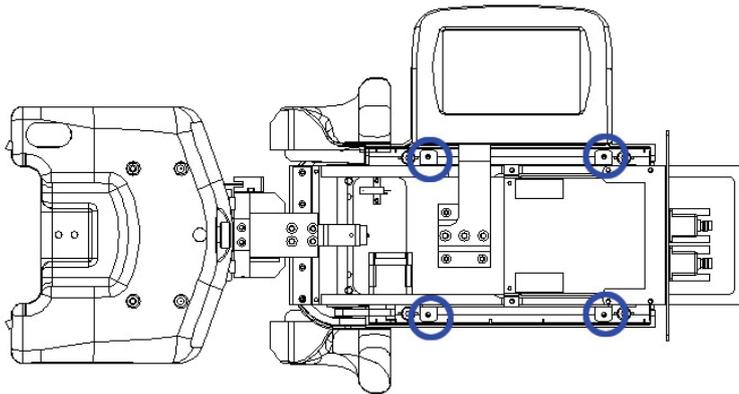
6. Remove 4 bolts, and then disassemble Case F.
