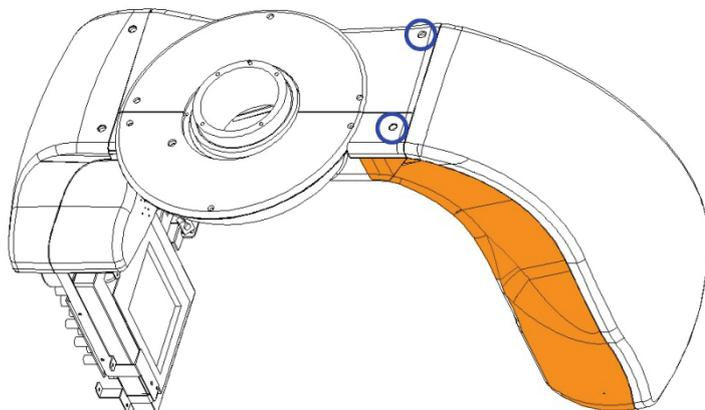
8. Remove 2 bolts, and then disassemble Case C.
