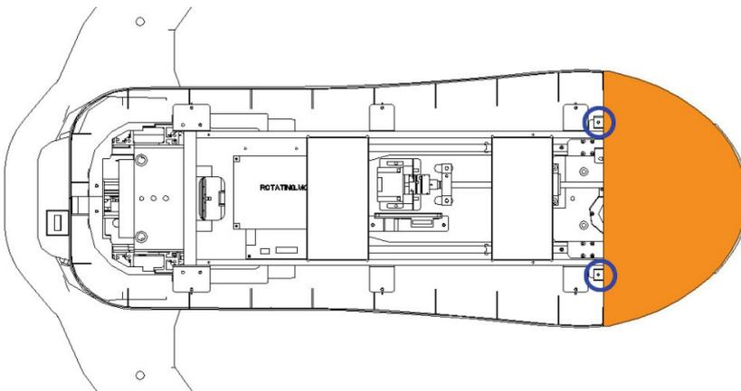
8. After removing 2 bolts, disassemble case G.
