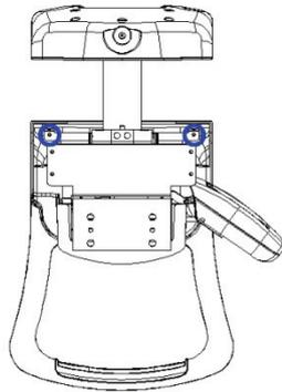
5. Remove 4 bolts, and then disassemble Case D.
