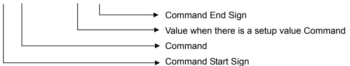
Example: **[SPM\_HV\_\_0800]**: Tube Voltage Setting Command
