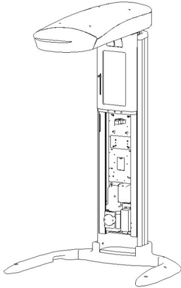
4. Remove 4 bolts, and then disassemble Case E.
