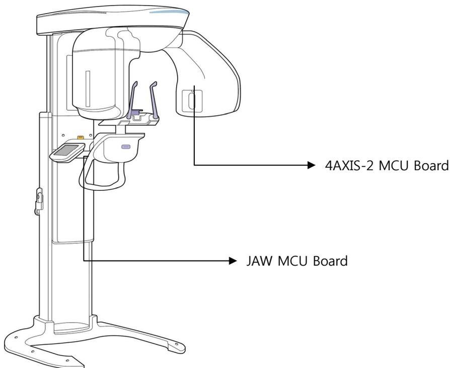
**4AXIS-2 MCU** and **JAW MCU** Boards use **EzCAN (Version: 1003)** program to implement the firmware upgrade.
