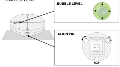
Put CT NUMBER CHECK PHANTOM on the PHANTOM JIG ASS'Y.
