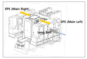
5. Pull out the Main Unit with the EPS (Main Base).from the pallet.
