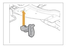
2. Connect the UP/DOWN switch to the unit and hang it on the UP / DOWN Switch Holder
