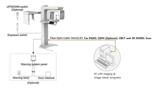
Fiber Optic Cable - Used to transfer image data to the PC.
