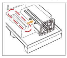
2. Assemble the upper carrying handle by using one wrench bolt.
