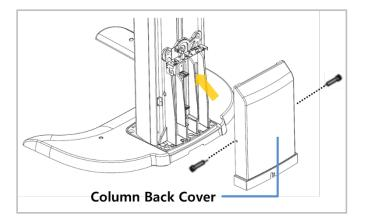
3. Ensure the cables go through the Column Back Cover holes as shown in the figure.
