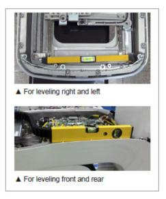
5. Turn each set screw clockwise or counterclockwise to make the equipment level while another person monitors the level indicator.
