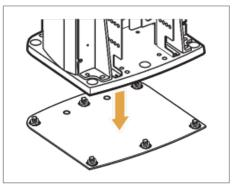
4. Put the washers and nuts into the six anchored bolts on the floor and tighten the nuts loosely. Make sure that you put the fasteners in the sequence, as shown in the figure.
