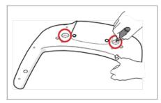
2. Drill the floor holes of size 12 mm x 30 mm (depth) using the concrete hammer drill.
