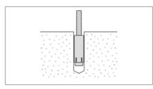
5. Secure the anchor bolts with the hammer.
