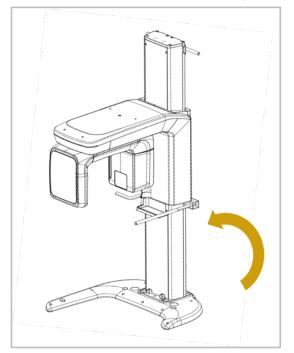
6. Put the equipment in a vertical position slowly while holding the upper handle.
