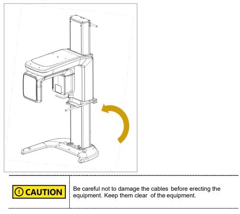
3. Put the Equipment on the aligning plate while making sure that the column bottom holes engage in the anchored bolts.
