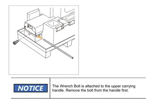
3. Assemble the lower carrying handle by using two Wrench Bolts.
