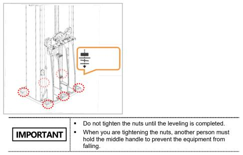
5. Installing the Equipment: Wall Mount
