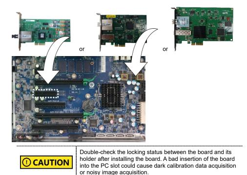
4. Put the slot holder back to its initial position.
