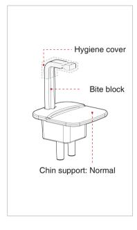
A. Insert the normal chin support and bite block into the chin support receptacle on the equipment.
