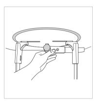
C. The nasal positioner should be flipped to the side and upward to prevent it from obstructing the image acquisition.
