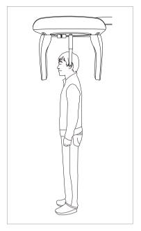
E. Adjust the height of the unit to suit the patient by pressing the column up / down button or switch (optional).
