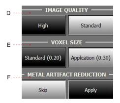
D. Select the image acquisition speed under High (24 s) or Standard (15 s).
