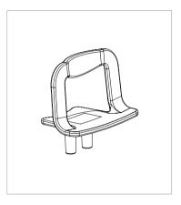
A. Insert the chin support (Sinus) into the receptacle on the equipment.
