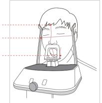
B. Frankfurt plane laser beam: Position the patient's head so that the Frankfurt plane is aligned with the Frankfurt plane laser beam.
