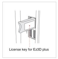
D. Insert the license key for Ez3D plus into the USB port on the back of PC. The license key for Ez3D plus must be attached to view or analyze the 3D images.
