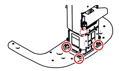
7. Remove the top carrying handle using an Allen Wrench.
