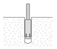
5. Secure the anchor bolts with the hammer.
