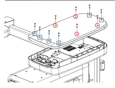
4. Put two Silicon caps on the bolt's top connecting the Joint Bracket.
