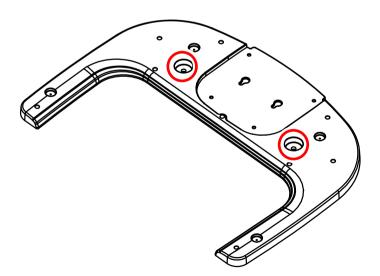
2. Drill the floor holes of size 12 mm x 30 mm (depth) using the concrete hammer drill.
