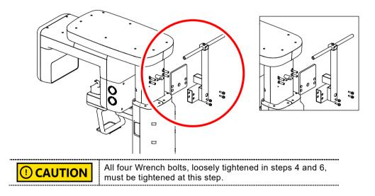
8. Loosen the four bolts with an Allen Wrench and remove the part attached to the Column.
