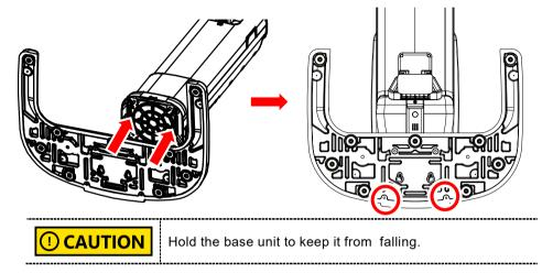
4. Tighten them with an Allen Wrench to connect the Base Unit to the Column Unit.
