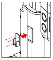
3. Attach a sticker on the other side of the equipment where you did not install the UP/DOWN Switch Holder
