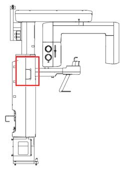
2. Assemble the UP/DOWN Switch Holder: Insert three Truss Bolts into holes on the holder (see below) and tighten them with a crosshead screwdriver until they no longer move.
