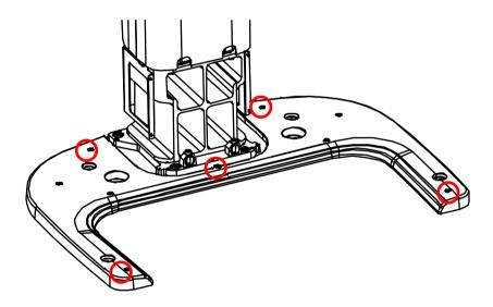
3. When leveling the equipment is completed, ensure to tighten all eight Screws until they no longer move.
