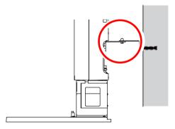
2. Tighten the nuts in the anchored bolts.
