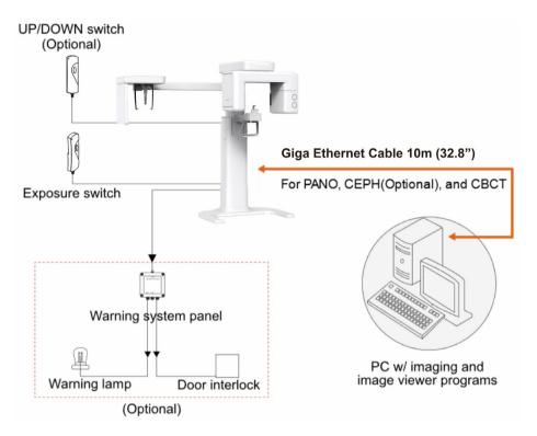
Giga Ethernet Cable - transfers image data to the PC.
