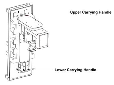
2. Put the main unit with the EPS (Main Base) on a Transport Dolly and move it to the installation site.
