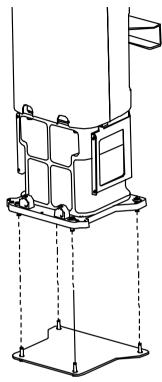
4. Place the washers and nuts on Anchor Bolts. Tighten each nut loosely with a fastener.
