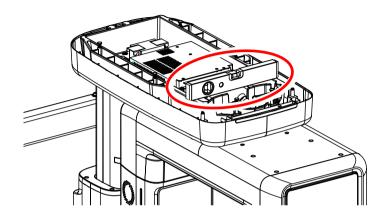
2. Turn Screws in marked locations left and right until the Sprit Level bubble comes to the center.
