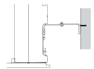
Tighten two bolts conjoining the column and wall brackets.
