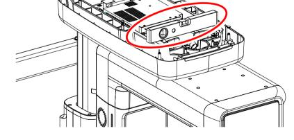
5. Place the Spirit Level on the Vertical Frame, as shown in the following figure.
