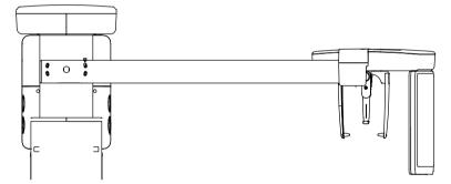
3. Put the four wrench bolts into each hole and tighten with an Allen Wrench to fix the CEPH arms on the Main Unit.
