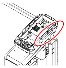
2. Turn Screws in marked locations left and right until the Sprit Level bubble comes to the center.
