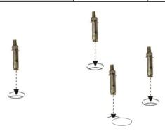
4. Using the hammer, insert an EHS tool into the inner bolt.
