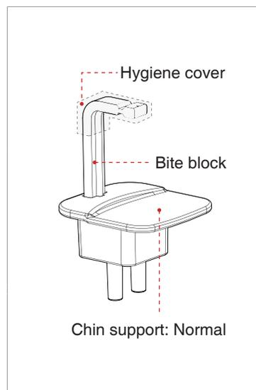
A. Insert the normal chin support and bite block into the chin support receptacle on the equipment.
