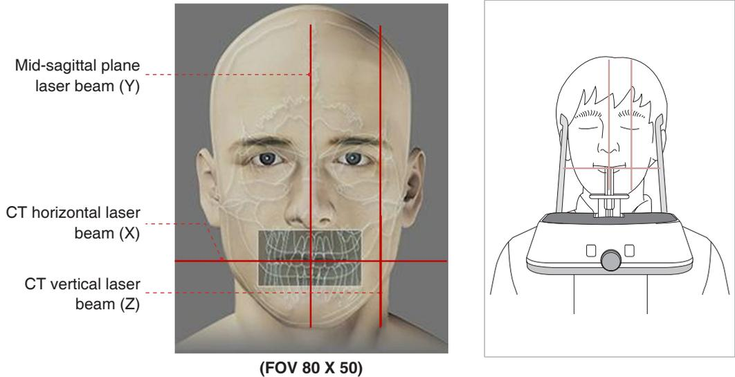
**A. CT horizontal laser beam (X):** Position the CT horizontal laser beam at the center of the FOV area. If necessary, the CT horizontal laser beam can be manually adjusted by pressing the Chinrest up / down button to make fine adjustments (① → ② → ③).
