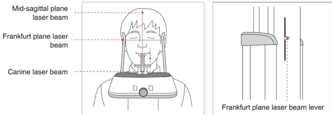
**C. Canine laser beam:** Have the patient smile to properly position the canine laser beam on the center of the patient's canine tooth. Rotate the thumb wheel, located under the patient support rest, forward or backward to properly align the beam.
