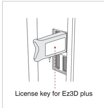
D. Insert the license key for Ez3D plus into the USB port on the back of PC. The license key for Ez3D plus must be attached to view or analyze the 3D images.
