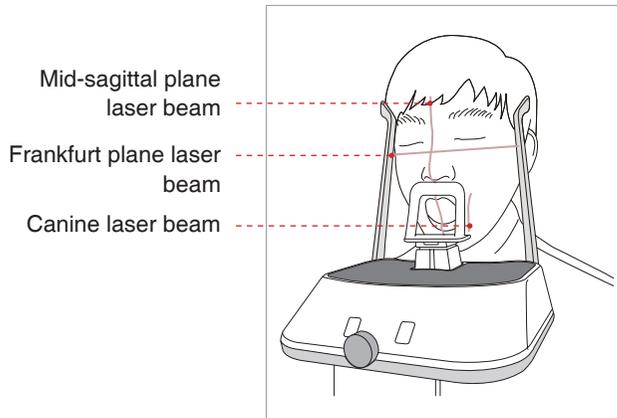
**B. Frankfurt plane laser beam:** Position the patient's head so that the Frankfurt plane is aligned with the Frankfurt plane laser beam.
