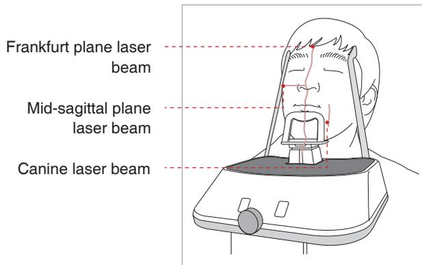
**A. Mid-sagittal plane laser beam:** Position the Mid-sagittal plane laser beam at the center of the patient's face to prevent magnifications of the left or right side in the final image.
