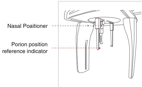
A. Turn the ear rods 90° clockwise from their initial position as shown in the illustration.
