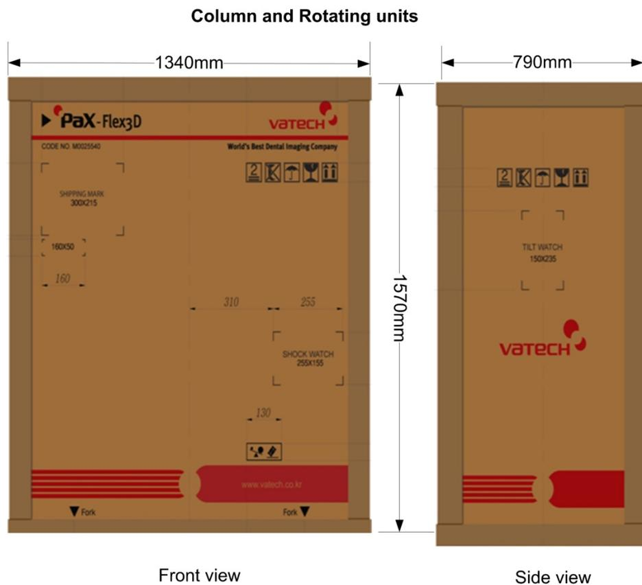
2. Move this carton near the installation site and open the top cover of the carton.
