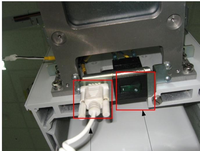
1. Connect the UP/DOWN switch, as shown in left figure
