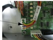
3. Connect MCU CN19 cable into the CN19
