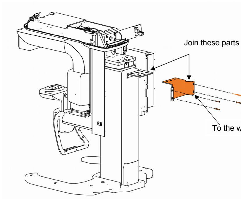
3. The following figure shows the 3-dimensional view after the floor anchors and wall mount bracket are installed.
