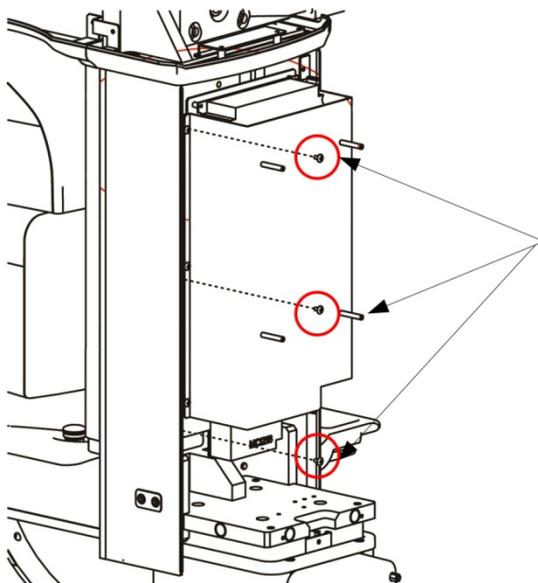
4. Tighten three truss bolts(M4 x8)
