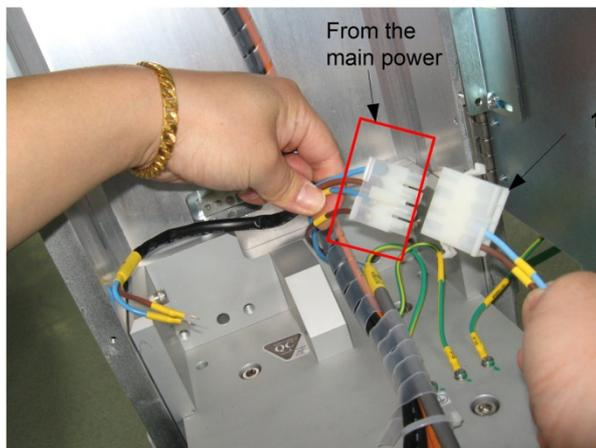
2. Connect the cable **18A** with the main power supply
