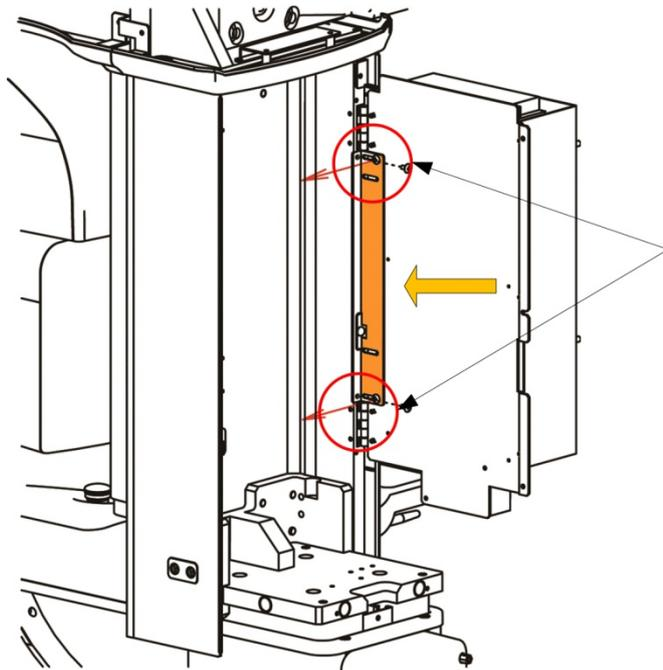
1. Loosen these two screws to make the bracket movable
