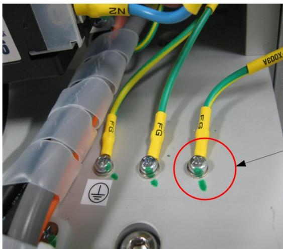
3. Fasten this ground cable onto the frame firmly to make perfect contact
