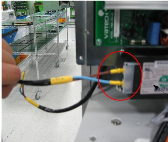
2. Connect firmly two ends of wires
