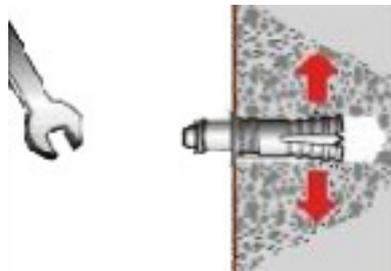
5. Attach and tighten the wall bracket (**Part No. 40**) to the wall, with the anchor bolts (**M8: Part No.:40**).
