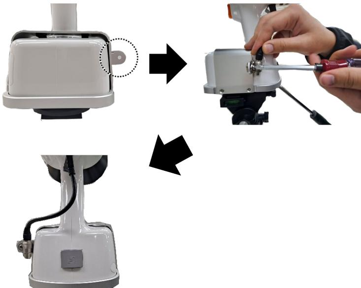
7. Connect the Remote X-ray Exposure Switch to the Gender Cable.
