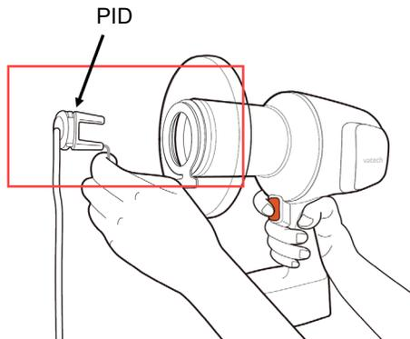
When using the PID, the X-ray device's exit pattern should be aligned perpendicular to the target receptor, as shown in the following figure.
