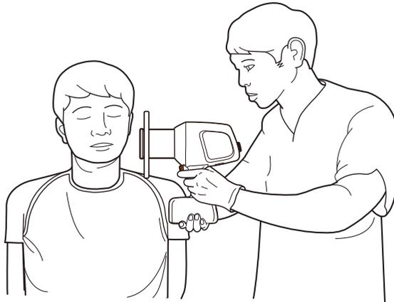
If you are in a country that does not allow using a hand-held X-ray in the clinic, use the device with a tripod, base holder, and remote exposure switch. To learn the proper use of each of these components, see **4.5.1 Remote Exposure Switch** and **A.1 How to Attach a Device to a Tripod**.
