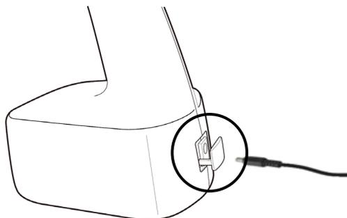
2. When the battery charger is connected, the battery charging LED indicator light comes on. Charge the battery until all the three LED indicators are filled up.
