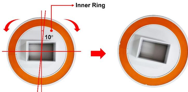
1. Assemble the Rotating Rectangular Cover to the Cone of the Main body.
