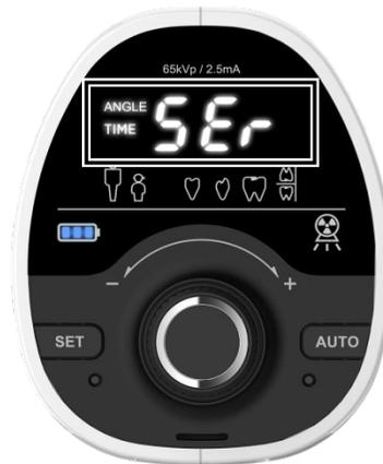
5. The system provides **24** service modes. To change each mode's settings from **n.01** to **n.24**, press the **AUTO** button on the left. Upon pressing the button, n.01 is displayed on the control panel.
