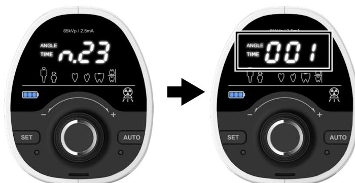
2. To turn off the Power Down Mode, turn the dial to change the setting from **"001"** to **"000"**.
